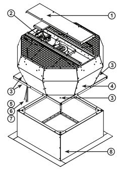
Fig. 2: Assembly size DVA...EC C
